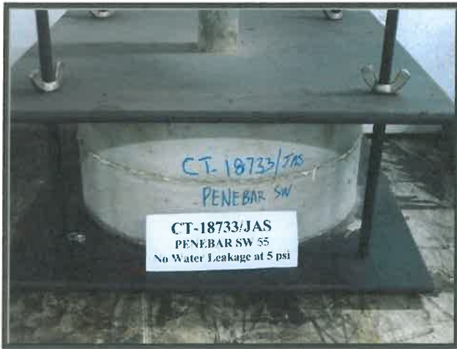
Photograph 3: Treated Sample at 5 psi water pressure
