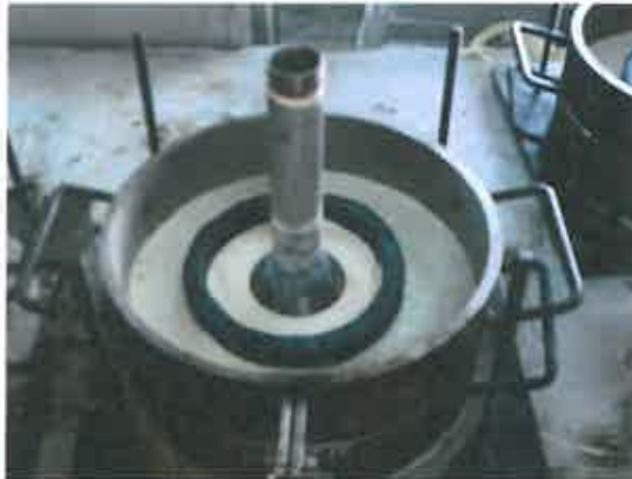
The PENEBAR SW-55 waterstop glued with PENEBAR SW Primer onto the bottom test specimen and the circular funnel with the pipe. A steel form of 80mm in height was clamped onto the bottom test specimen to be filled up with fresh concrete.
