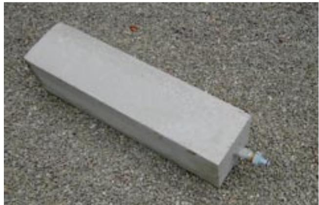
A pre-mixed concrete type of the quality C 16/20 has been used. After 28 days of curing the bars have been placed in a concrete testing machine and pressure was applied as much as necessary so that the bar broke and a crack has been formed.
