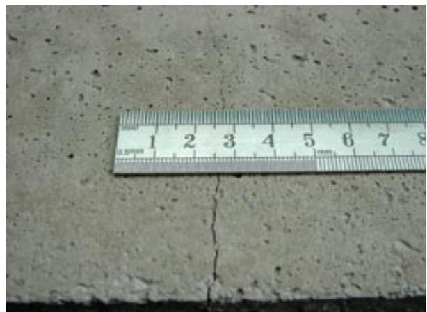
To test the water-permeability the hollow space has been filled with water each 24 hours. By permanent refilling the flow-out through the crack within 15 minutes has been determined. The samples 1 and 6 (marked with \*) have been connected to the water-pipe and a permanent water flow of 215 ml/min (measured at free flow out) has been adjusted. The following pictures show the situation.
