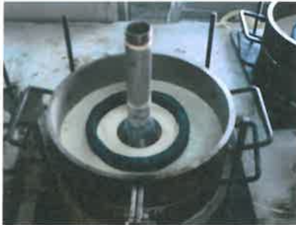
The PENEBAR SW-55 waterstop glued with PENEBAR SW Primer onto the bottom test specimen and the circular funnel with the pipe. A steel form of 80mm in height was clamped onto the bottom test specimen to be filled up with fresh concrete.
