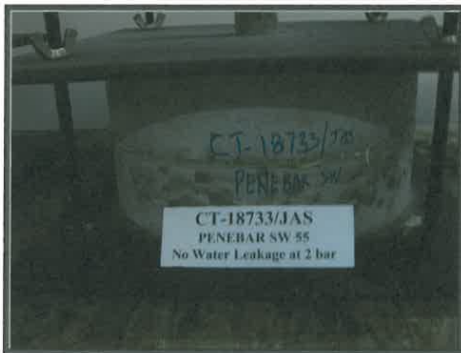
Photograph 6: Treated Sample at 2 bar water pressure
