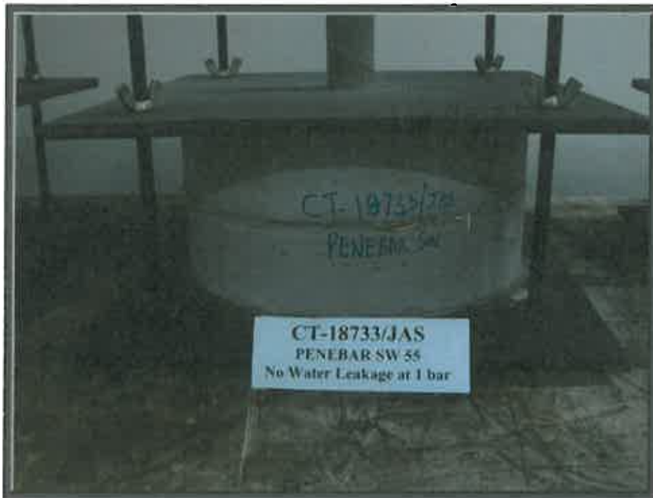
Photograph 5: Treated Sample at 1 bar water pressure
