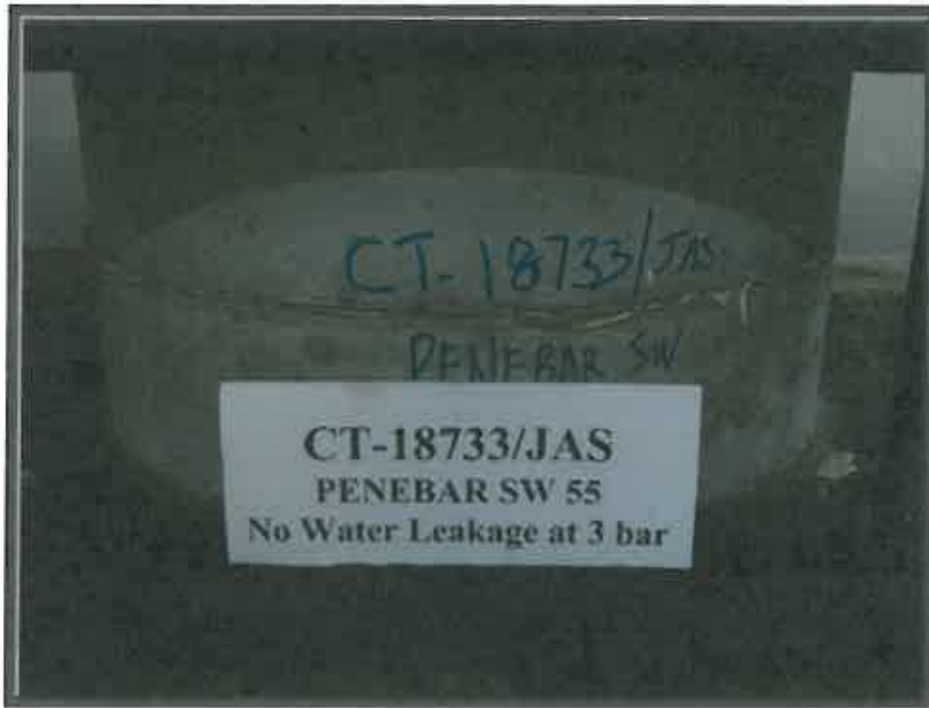
Photograph 7. Treated Sample at 3 bar water pressure
