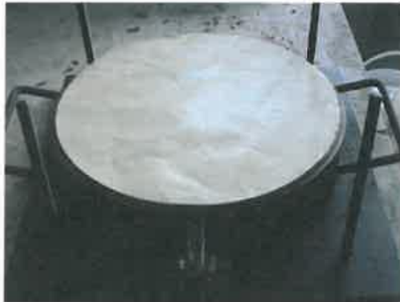
The release paper placed onto the control bottom test specimens
