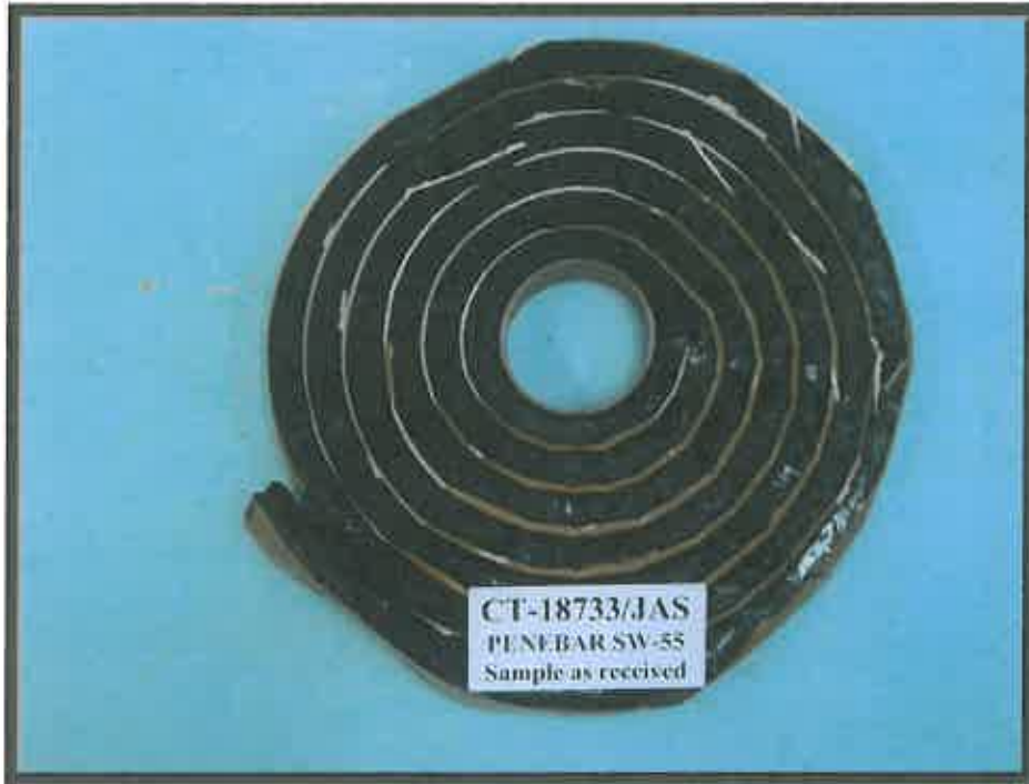
Photograph 1: Shows one roll of PENEBAR SW-55 waterstop as received
