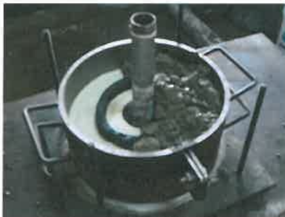
Fresh concrete placed onto the PENEBAR SW-55, release paper and the bottom test specimen
