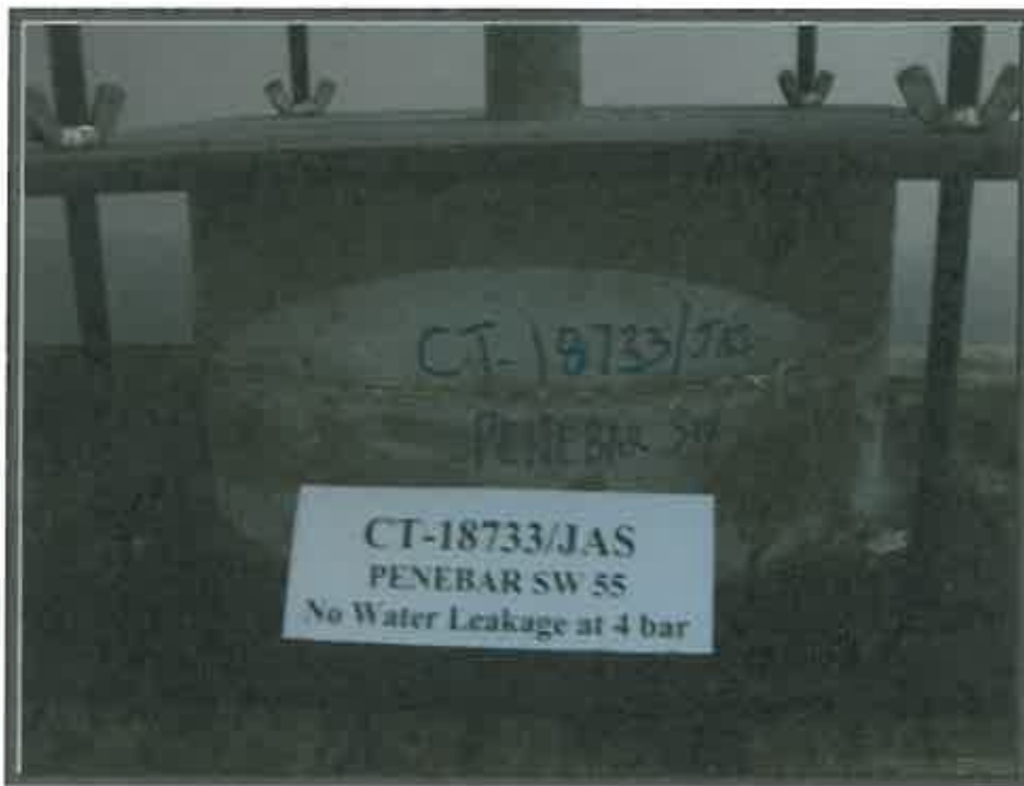
Photograph 8: Treated Sample at 4 bar water pressure
